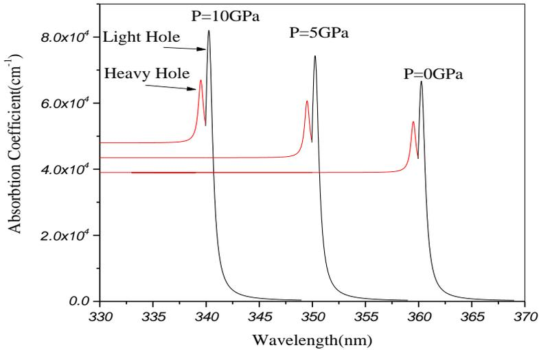
**Fig. 8.** Absorption coefficient for p-GaN-i(Al<sub>0.3</sub>Ga<sub>0.7</sub>N/GaN MQWSC)-n-GaN versus different hydrostatic pressure
