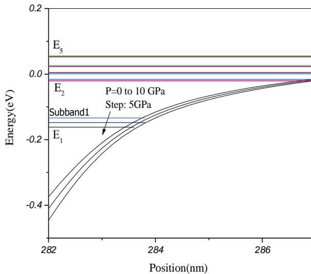
**Fig. 4.** The quantum well conduction band and subband of energy as a function of the distance under different hydrostatic pressure.
