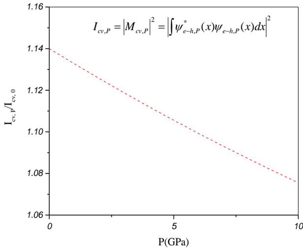
**Fig. 6.** Normalized square of the overlap of the electron–hole wave functions versus hydrostatic pressure.
