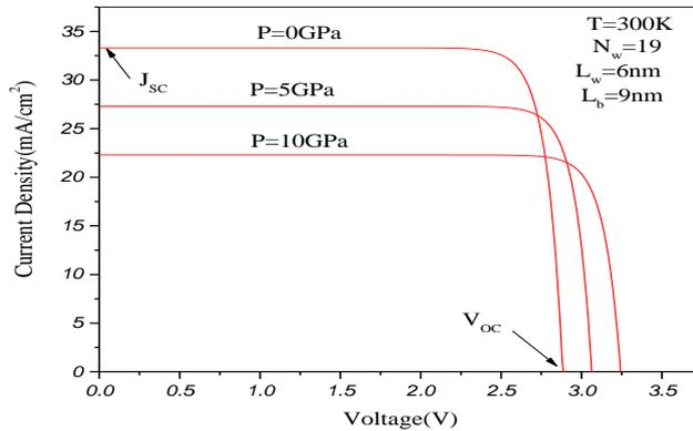
**Fig. 9.** Current-voltage characteristic of 20-MQW Al<sub>0.3</sub>Ga<sub>0.7</sub>N/GaN solar cell for various hydrostatic pressure.
