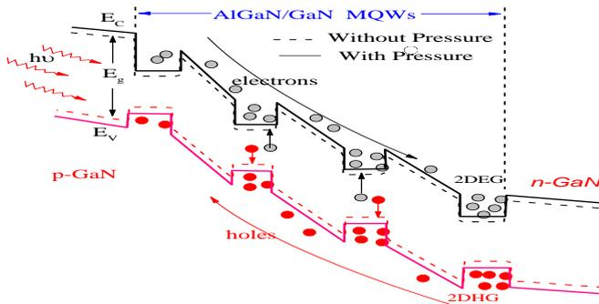
**Fig. 1.** Schematic profile of pGaN-i(AIGaN/GaN MQWSC)-n-GaN.
