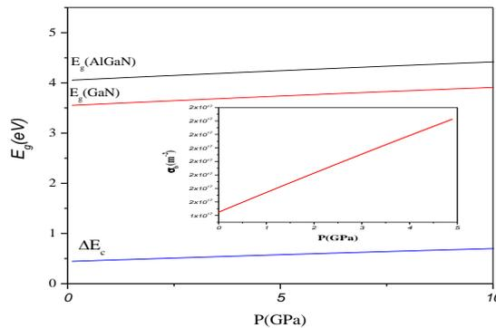
**Fig. 2.** The band-gaps energy of  $Al_{0.3}Ga_{0.3}N$ , GaN and conduction band offset of the  $Al_{0.3}Ga_{0.3}N/GaN$  as a function of pressure and temperature. The insert indicates the variations in the  $\sigma_b$  versus pressure
