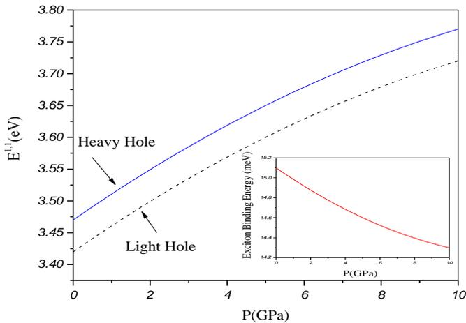
**Fig. 7.** The separation between the valance and conduction subbands ( $E_{CV}^{1,1}$ ) versus hydrostatic pressure. The insert indicates the exciton binding energy versus pressure
