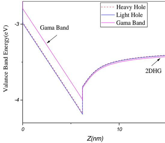
**Fig. 5.** Valence bands energy (Gamma, light and heavy holes bands in the vicinity of 2DHG) versus distances for  $\text{Al}_{0.3}\text{Ga}_{0.7}\text{N} / \text{GaN}$  heterostructure.
