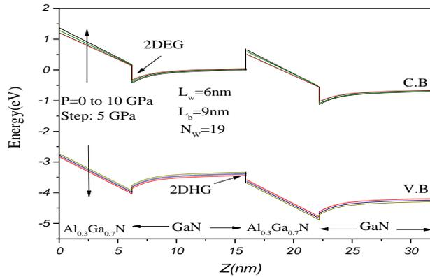
**Fig. 3.** The conduction(C.B) and valance(V.B) bands energy of  $\text{Al}_{0.3}\text{Ga}_{0.7}\text{N}/\text{GaN}$  hetrostructure as a function of the distance under different hydrostatic pressure.
