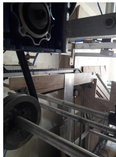
Fig. 1 A photo of the drive belt and pulley of the device
