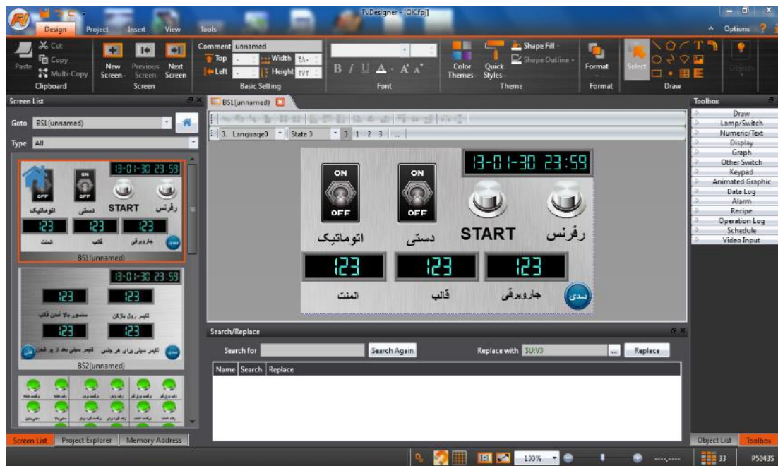
Fig. 8 Diagram of FvDesigner software for HMI programming
