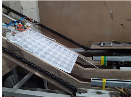
Fig. 4 Conveyor belt with height difference from the production surface
