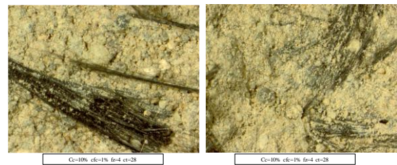
Fig. 13. Optical micrograph images of 28-day samples with 10% cement and 1% carbon fibers subjected to 4 freeze-thaw cycles.
