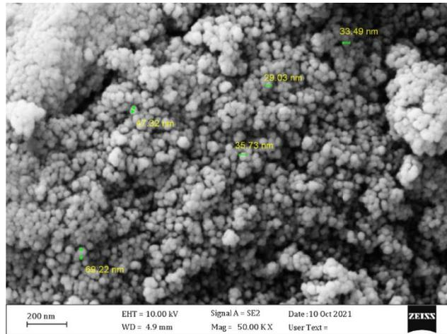
**Figure 2.** FESEM image of magnetite/nanocellulose particles.
