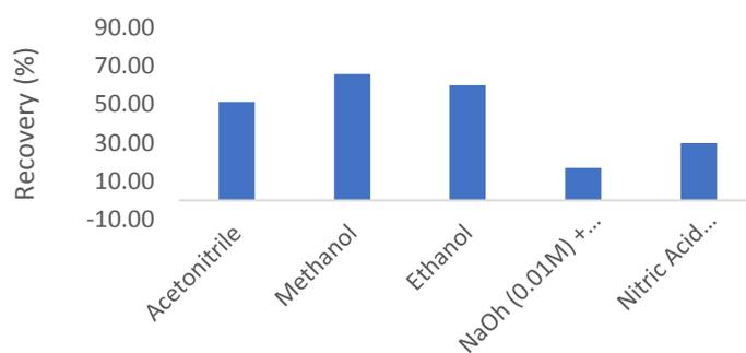
**Figure 19.** Examining the effect of different types of solvent and absorption.
