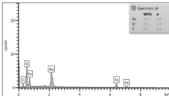
Figure 5. EDS analysis of magnetite/nanocellulose sample.
