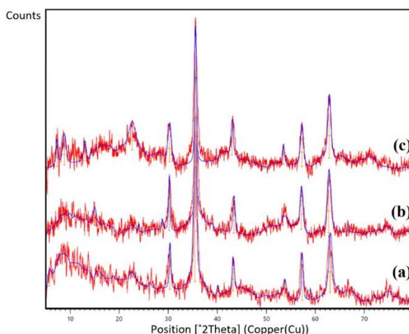
**Figure 1.** a) XRD spectrum of magnetite/nanocellulose b) XRD spectrum of magnetite/nanocellulose/betacyclodextrin c) XRD spectrum of magnetic nanoabsorbent with theophylline drug.
