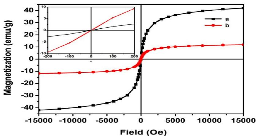
Figure 8. a) VSM diagram of magnetite b) VSM diagram of magnetite/nanocellulose/betacyclodextrin.
