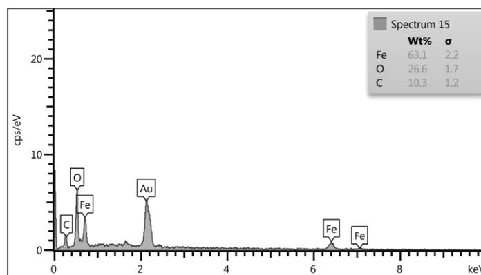
**Figure 6.** EDS analysis of magnetite/nanocellulose/betacyclodextrin sample.
