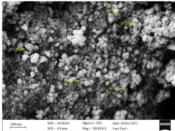
**Figure 3.** FESEM image of magnetite/nanocellulose/betacyclodextrin particles.
