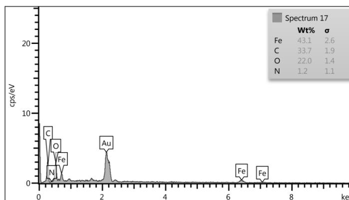
**Figure 7.** EDS analysis of magnetite/nanocellulose/betacyclodextrin magnetic nanoabsorbent sample with theophylline drug.
