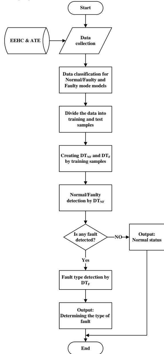
Fig. 1. Proposed method for detecting power transformer faults.
