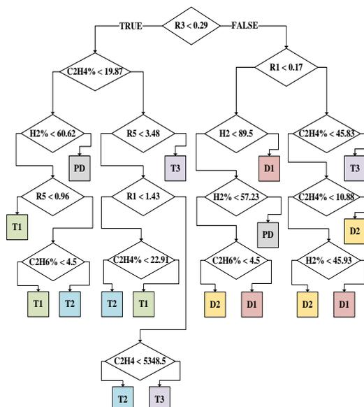
Fig. 9. Final DTF: Identifying the type of fault.
