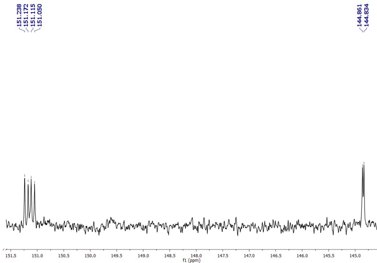
Figure 6. ^{13}\text{C}\{^1\text{H}\} NMR spectrum of (\text{C}_6\text{H}_5\text{O})_2\text{P}(\text{O})[\text{NH}-(S)-(-)\text{CH}(\text{C}_2\text{H}_5)(\text{C}_6\text{H}_5)] in the range of 144 to 152 ppm. The two doublets within 151.05 to 151.24 ppm are related to the diastereotopic ipso -carbon atoms. The doublet at 144.85 ppm is related to the phenyl ring of chiral amine.
