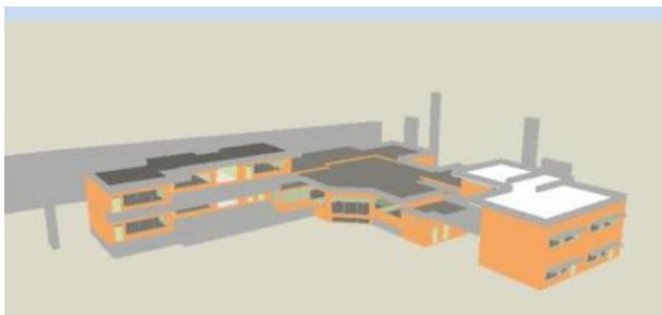
Fig 5: the location of the cool roof of the north and southeast classroom, the northern staircase, and the classroom adjacent to the northern staircase
