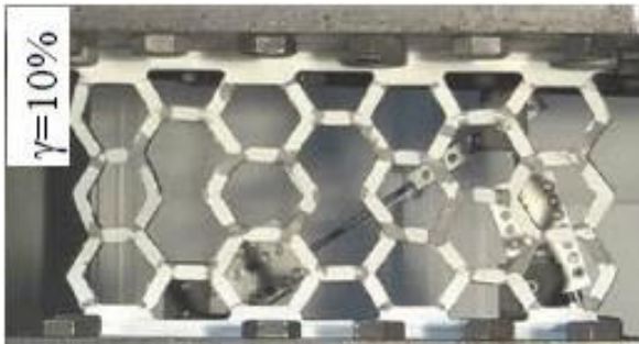
Fig. 9. Deformation after loading in HSF experimental specimen [17]
