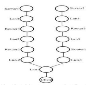
Figure (2): Logical topology corresponding to Figure 1.
