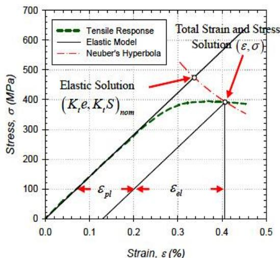
Fig. 2 The Application of Neuber method for determination of notch root stress and strain [9]
