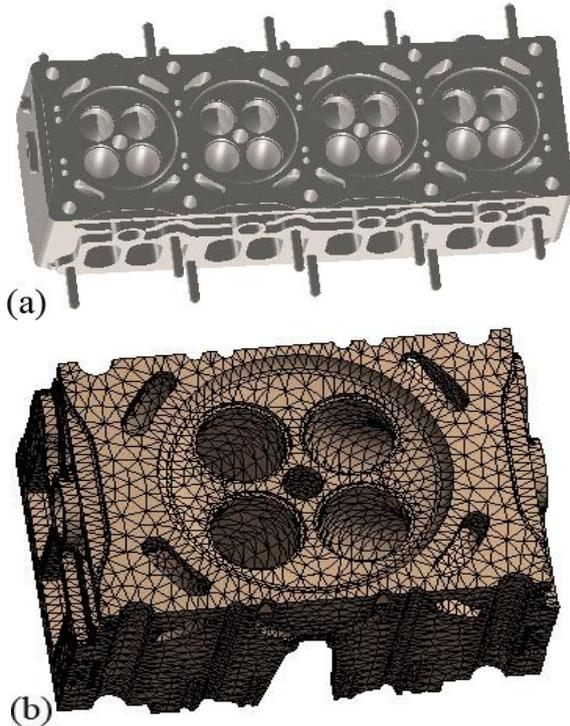
Fig. 1 (a) The cylinder head generated by SolidWorks, (b) Finite element model of the cylinder head
