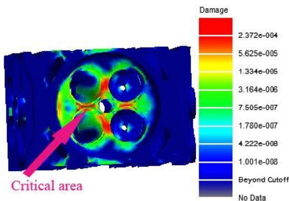
Fig. 9 The fatigue damage based on Morrow equation in the cylinder head
