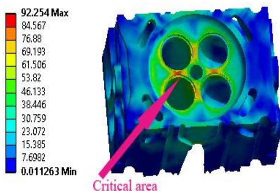
Fig. 5 The Von-Mises stress distribution in the cylinder head
