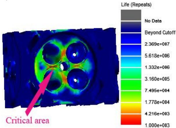
Fig. 8 The number of cycles to failure based on Morrow equation in the cylinder head
