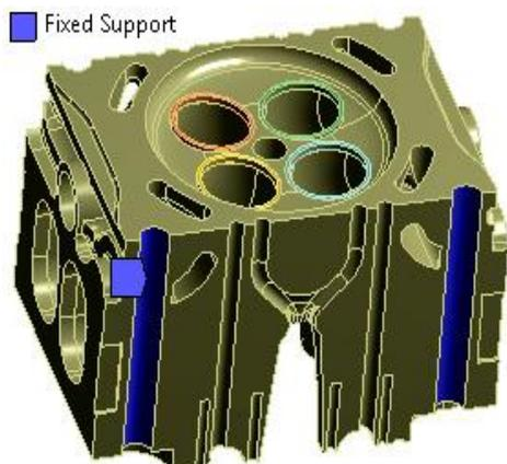
Fig. 4: Structural boundary condition
