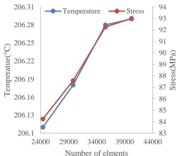
Fig. 7 The Temperature and Von-Mises stress versus number of elements
