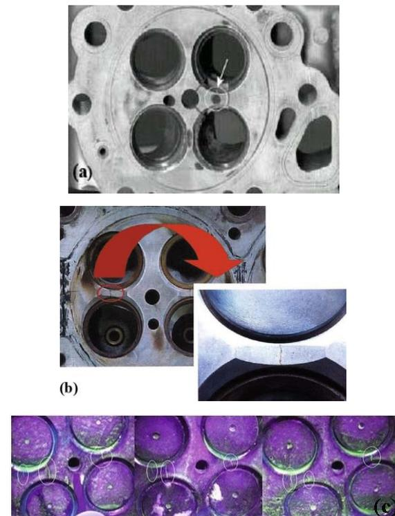
Fig. 10 The cracked cylinder head, a[30], b[31] , c[32]
