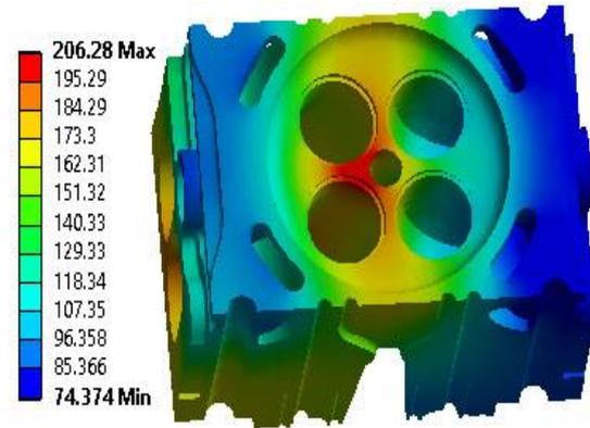
Fig. 3 The temperature distribution in the cylinder head
