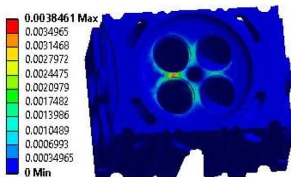
Fig. 6 The equivalent plastic strain distribution
