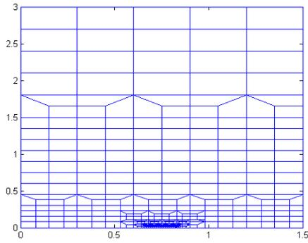
Fig. 3 Specimen idealizations in x-y plane
