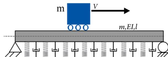
Fig. 1 Schematic of Beam-moving mass system
