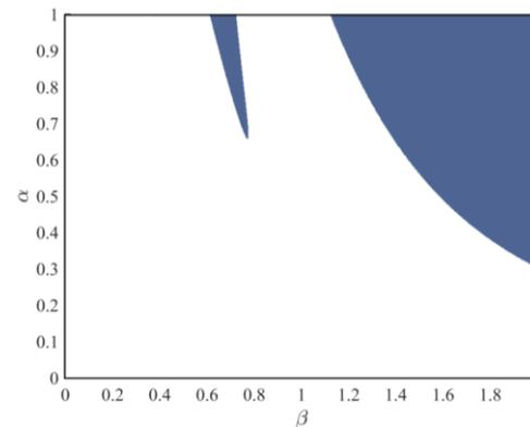
Fig. 2 Stability plane of beam with fixed-fixed boundary conditions
