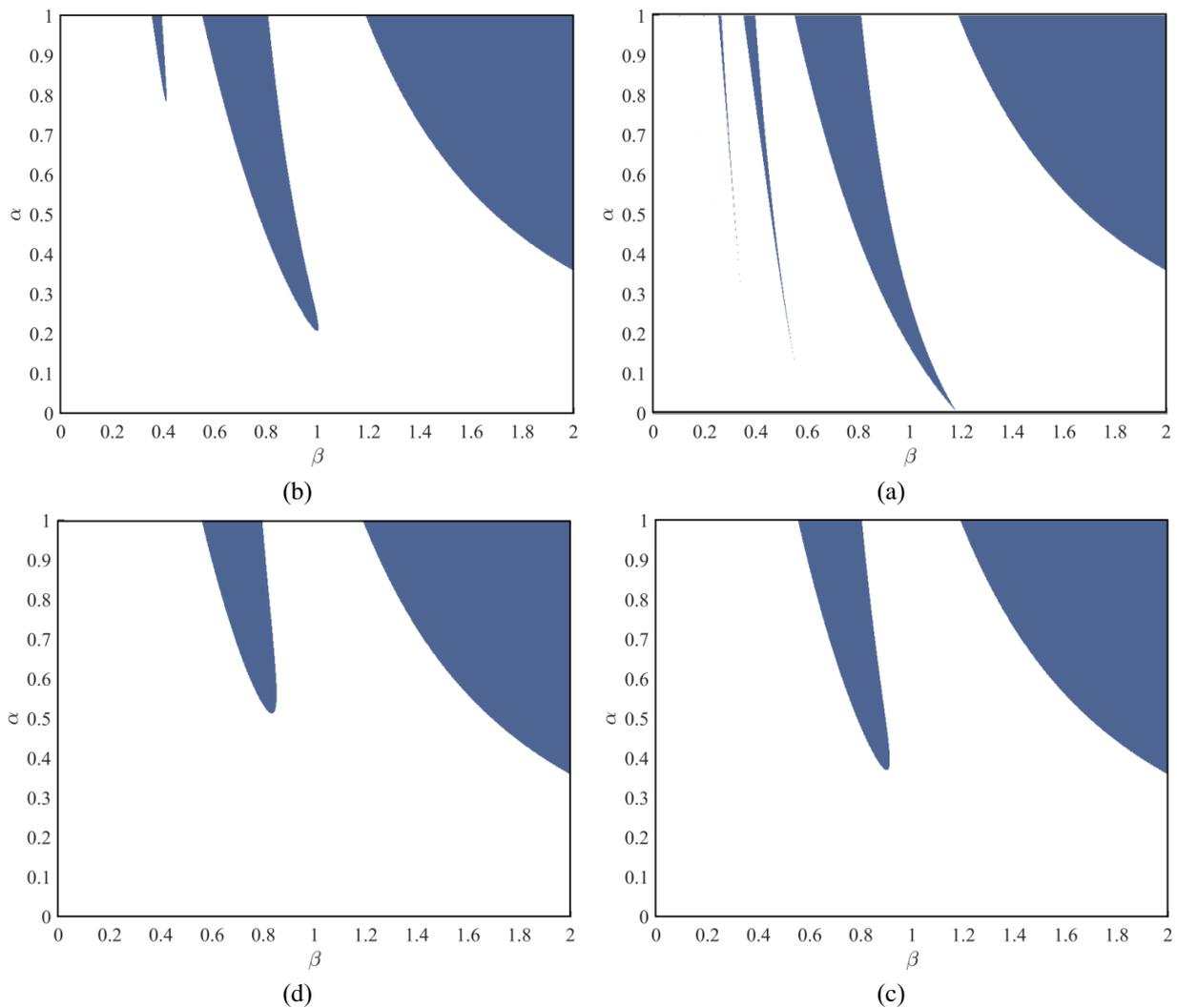
Fig. 5 the effect of damping on the stable and unstable regions of the simple-simple beam (a)  $c^* = 0$  (b)
