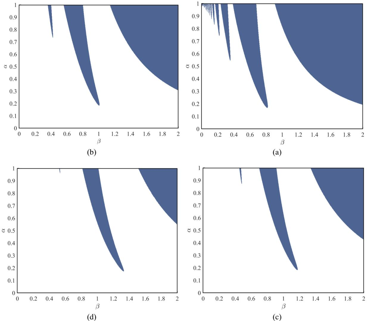
Fig. 4 The effect of the stiffness of the elastic medium on the stable and unstable regions for simple-fixed beam
