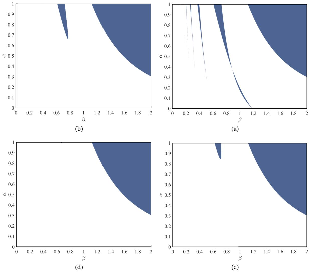
Fig. 6 the effect of damping on the stable and unstable regions of the fixed-fixed beam (a)  $c^* = 0$  (b)  $c^* = 0.1$  (c)  $c^* = 0.2$  (d)  $c^* = 0.3$
