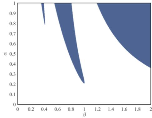
Fig. 1 Stability plane of beam with simple-simple boundary conditions
