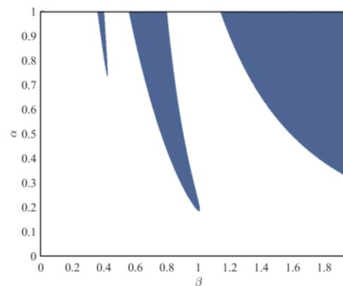
Fig. 3 Stability plane of beam with simple-fixed boundary conditions
