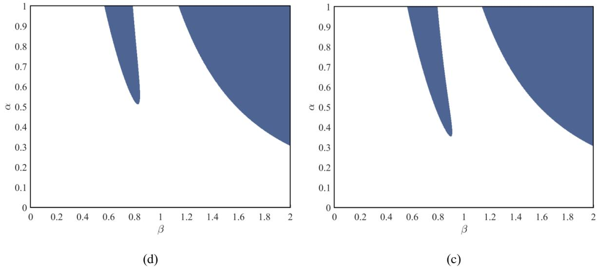
Fig. 7 the effect of damping on the stable and unstable regions of the simple-fixed beam (a)  $c^* = 0$  (b)  $c^* = 0.1$  (c)  $c^* = 0.2$  (d)  $c^* = 0.3$
