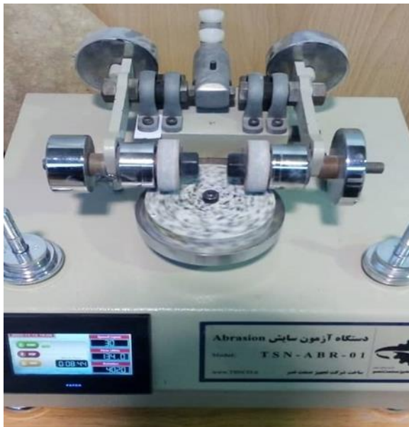
Fig. 2 Taber abrasion test machine.
