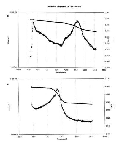
Fig. 4. DMTA Curves of copolymers: (a) III and (b) III<sub>ez</sub> 5 °C/min in air.
