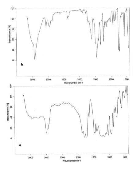
**Fig. 2.** Infrared spectra of: (a) II and (b)  $II_{ez}$ .
