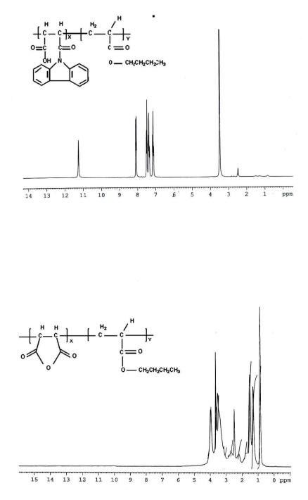
**Fig. 3.** <sup>1</sup>H NMR spectra: (a) V and  $V_{cz}$  in DMSO.
