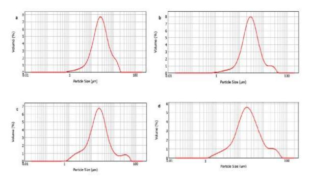
Fig. 1. Particle size distribution curve of pistachio paste produced using a Colloid mill at different gap size (a=20 µm; b= 40µm; c=60µm and d=80µm)
