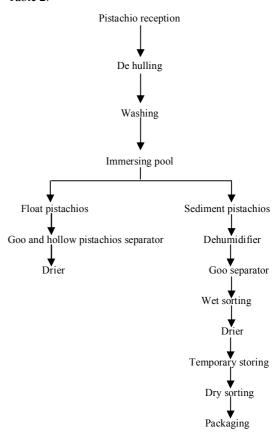
Fig 1. Process flow diagram
