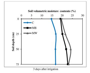
Fig. 5. The average changes in soil moisture content in different treatments between two consecutive irrigation in the orchard 2
