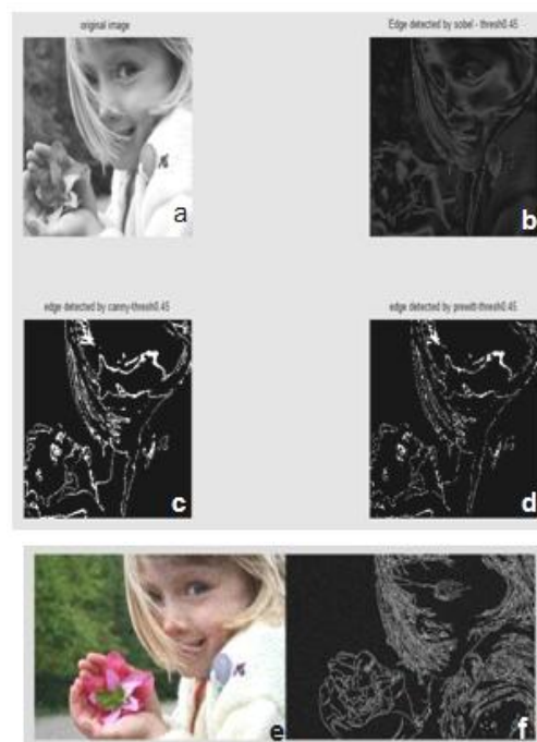
Fig.9. (a) original image (b) edge detected by Sobel(c) edge detected by canny (d) edge detected by Prewitt (e) salt paper noises image (f) edge detected by proposed method
