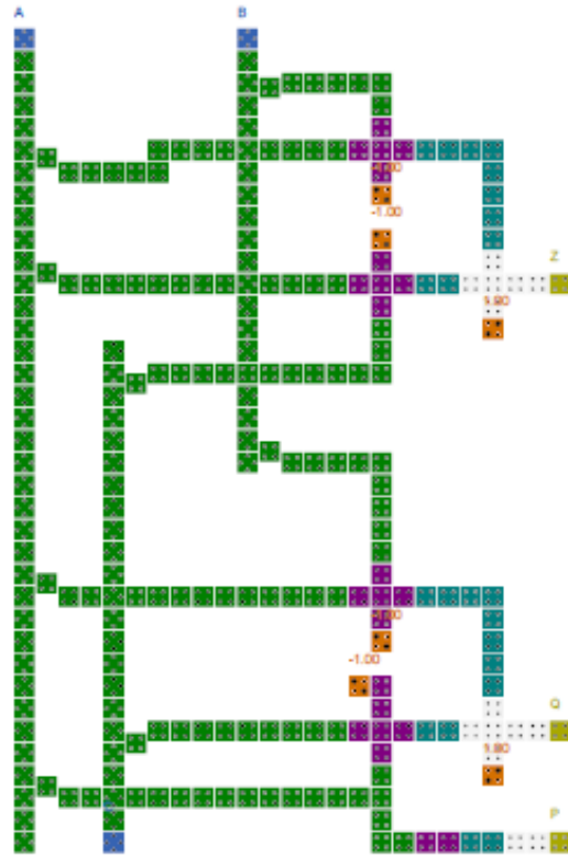
Fig. 11. Layout of testable Fredkin gate
