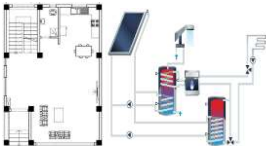
Fig. 3. Schematic of the SWH system and the investigated space
