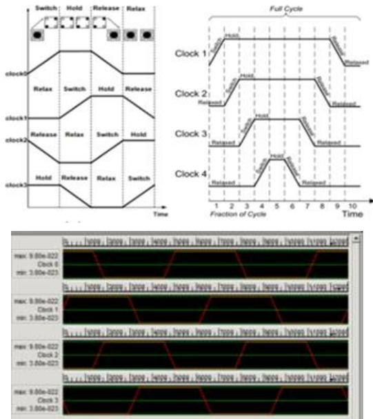
Fig. 3. QCA Zone clocking (a) Landauer clocking waveform [1] (b) Bennett clocking waveform [1] (c) clocking wave form in QCADesigner
