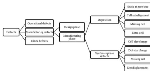
Fig. 5. Categorizing different defect types in QCA circuits
