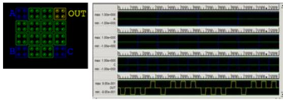
Fig. 12. Schematic and implementation of XOR and XNOR gates
