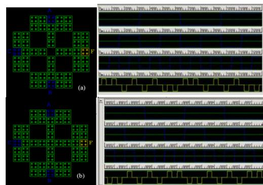
Fig. 9. Schematic, implementation, and simulation of XOR and XNOR
