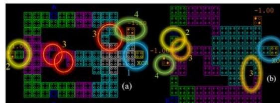
Fig. 16. XOR Defects that may occur in the two gates presented in [27] and [28]: 1- Poor output transmission, 2- Possibility of clock fault, 3- Possibility of bridging fault, 4- Possibility of stuck-at-0/1 fault.
