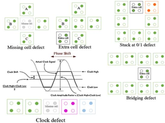
Fig. 6. A schematic diagram of the missing cell, extra cell defects in a majority gate and stuck at 0/1, clock [26] and bridging defects in a part of circuit
