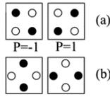
Fig. 1. A QCA cell (a) Position of electrons in a 90° cell (b) Position of electrons in a 45° cell
