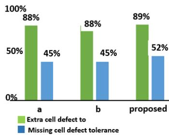
Fig. 17. XOR Comparing the tolerance of the proposed gates against defects with those of the gates presented in [27], [28] (shown in Figure 15)
