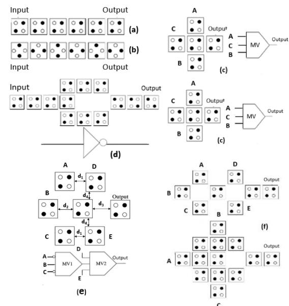
Fig. 2. Basic gates in QCA technology
