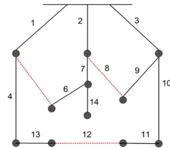
Fig. 2. 12-Node system initial grid construction
