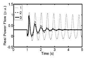
Fig. 9. Power flow response for a three-phase to earth short circuit at operating conditions (b)
