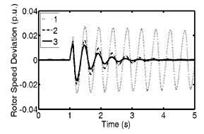
Fig. 8. . Rotor speed response for a three-phase to earth short circuit at operating conditions: (a)
