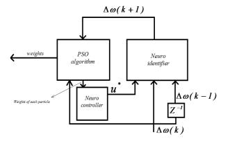
Fig. 2. Ttraining structure block
