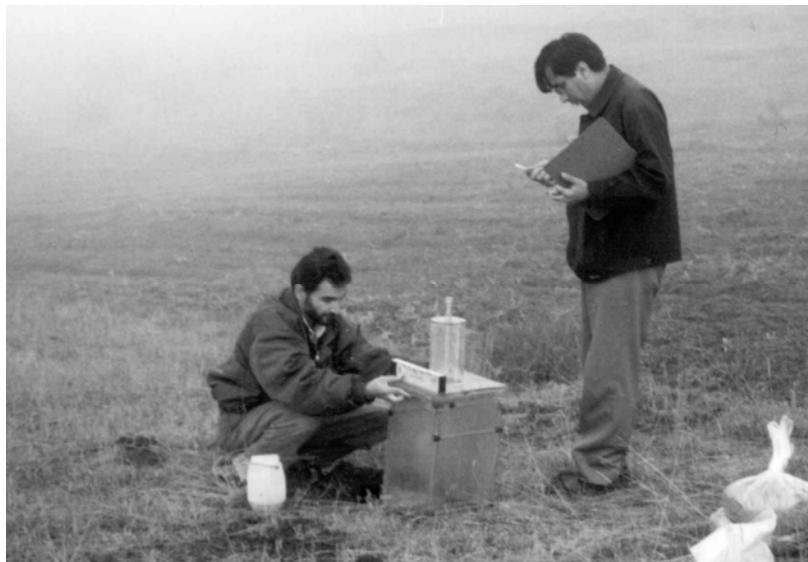
Fig. 3. View of Rainfall Simulator Used in This Study
