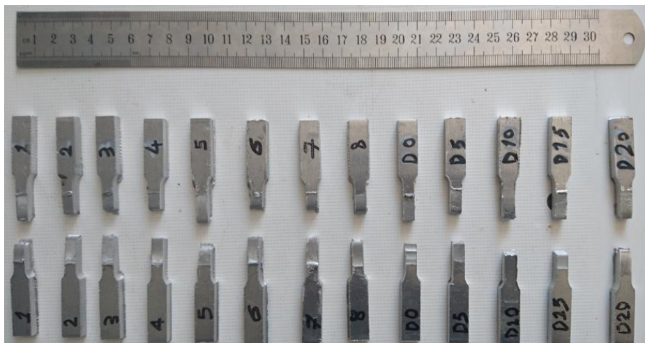
Figure 10. Several samples were deliberated after the tensile test
