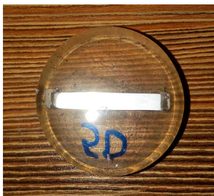
Figure 8: Schematic of a sample prepared for microhardness and microstructure tests
