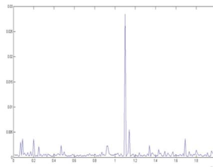
**Fig. 1.** *The maximum amplitude of PD in the case of DC voltages in oil-impregnated paper testing object*
