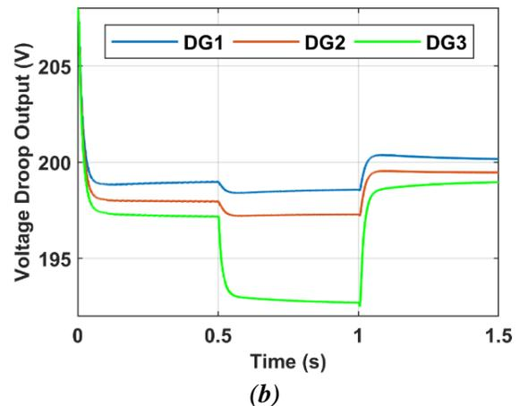
**Fig. 8. Output of temporal drop characteristics for  $m_p=0.00105 \times 1.5$ , (a) The output of the frequency drop characteristic, (b) Output characteristic of voltage drop.**
