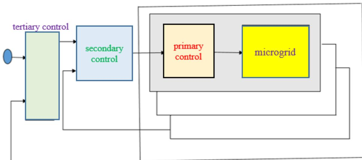
*Fig. 2. Hierarchical control system.*
