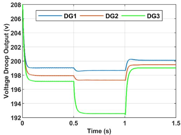
**Fig. 7. Output of the voltage drop characteristic of the sources using the usual drop strategy.**
