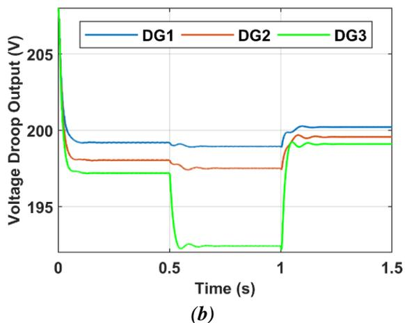
**Fig. 9.** Output of drop characteristics for  $m_p=0.00105 \times 5$ , (a) The output of the frequency drop characteristic, (b) Output characteristic of voltage drop.
