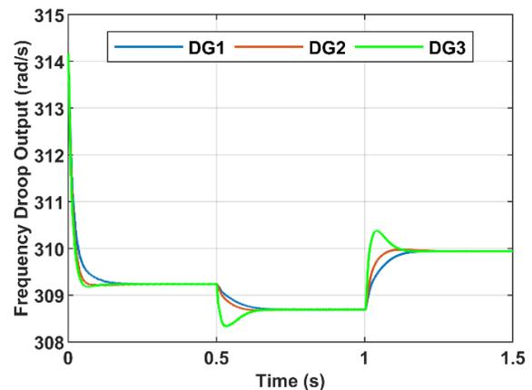
**Fig. 6. Output of the frequency drop characteristic of the resource using the usual drop strategy.**
