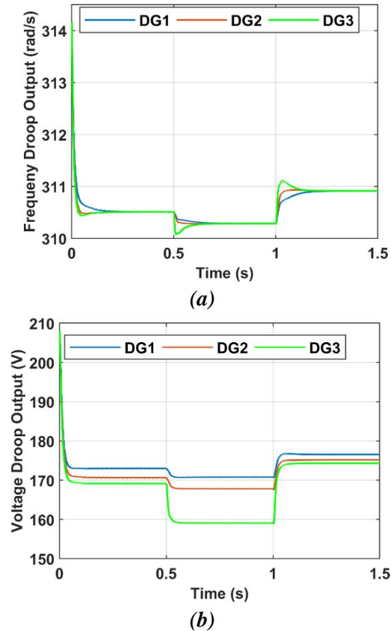
**Fig. 11. The output of the drop characteristics for  $n_q=0.0025 \times 5$ , (a) The output of the frequency drop characteristic, (b) Output characteristic of voltage drop.**
