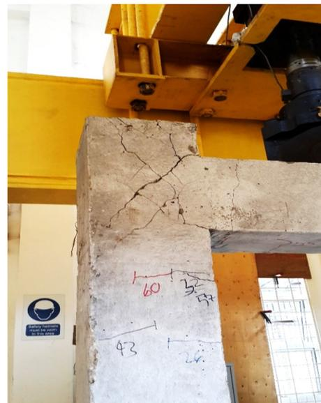
Fig. 8 Crack pattern on RCF
