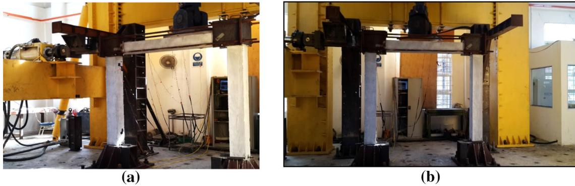
Fig. 5 Test setup: **a** frame with actuator on the left, **b** frame setup
