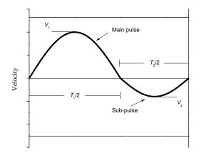
Figure 2. General form of a velocity pulse
