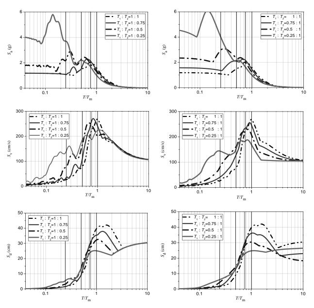
Figure 4. Acceleration, velocity, and displacement response spectra (amplitudes fixed, sub-pulse durations changing)
