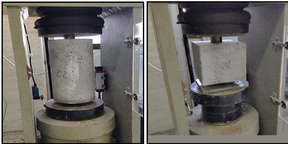
Figure 6. Cylindrical and cubic specimens under double punch test
