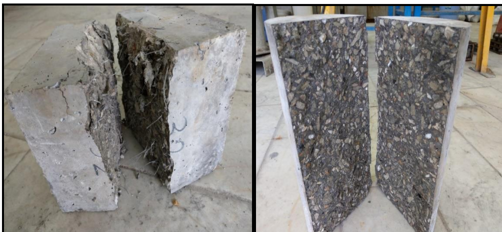
Figure 4. Cylindrical and cubic specimen broken in Barcelona test
