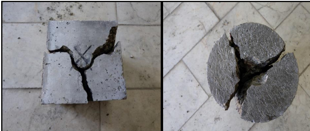
Figure 7. Cylindrical and cubic specimen is broken in double punch test
