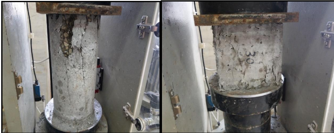
Figure 3. Compressive strength tests a) cylindrical sample b) cubic sample
