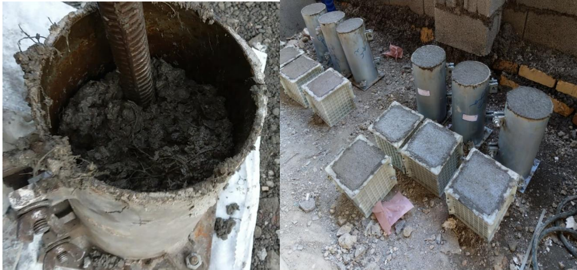
Figure 2. a) Compression in three layers b) Molded samples
