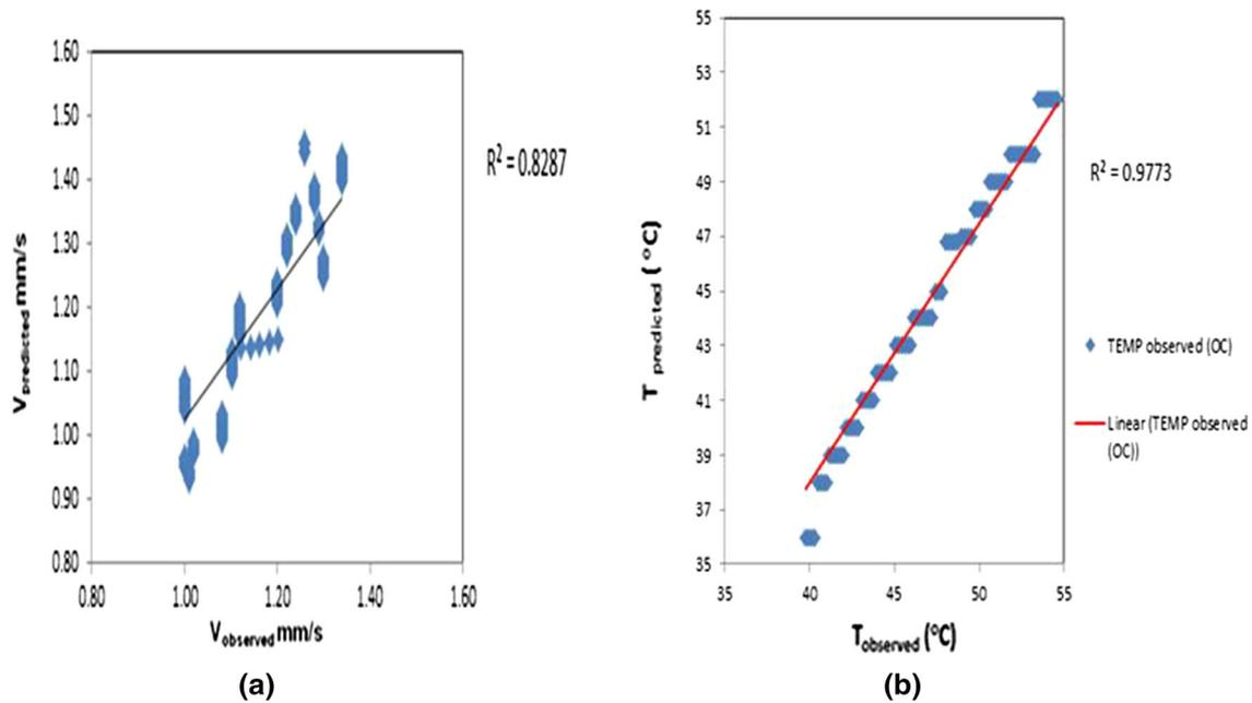
**Fig. 10** **a** Graph of vibration model validation, **b** temperature model validation
