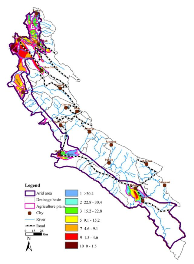
Fig. 4 Depth to water ranges and corresponding ratings according to DRASTIC model, in agricultural plains
