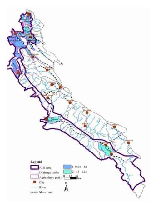
Fig. 10 Hydraulic Conductivity ranges and corresponding ratings according to DRASTIC model, in agricultural plains
