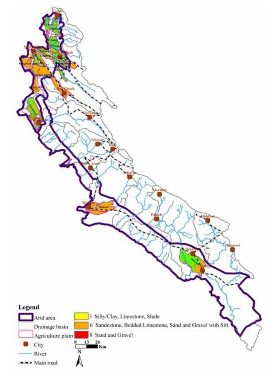
Fig. 9 The vadose zone media ranges and corresponding ratings according to DRASTIC model, in agricultural plains
