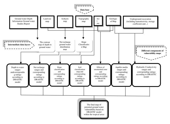
Fig. 3 The DRASTIC parameters rating method, from Aller (1987)
