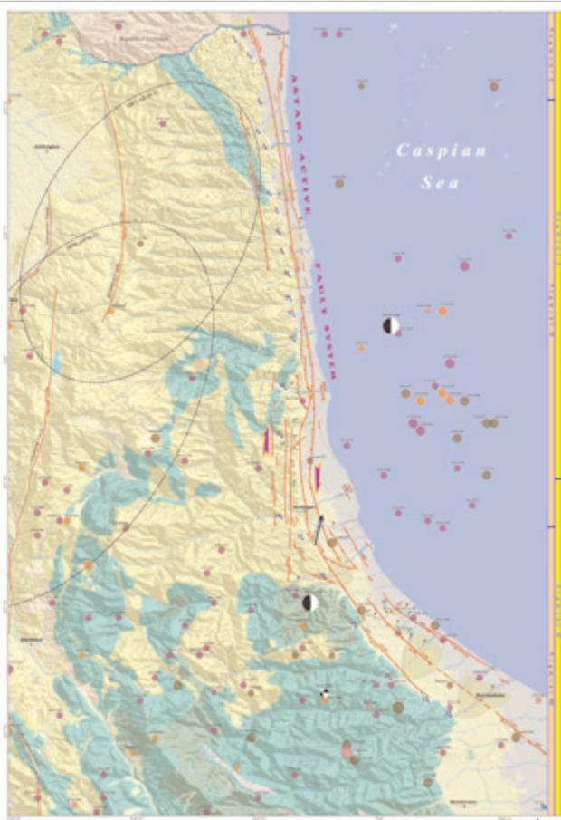
Figure 10. The fault system of Astarra on the basis of the map of Seismotectonics of Talesh heights and map simplified of geology, earthquakes displayed in the water area of west of the Caspian shows the structures of fold and the fault of growth of fault system of Astarra among deposits of sea context in the East, the colored columns of map side shows the segmentation of fault system of ATF and ASF based on the geometric changes (Kave Firuz et al. 2013).
