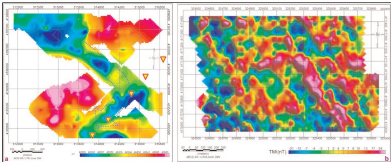
Figure 13. (a) data derived from geomagnetic perceptions in the region of Lavandevil, three corners show the location of the fault on the East of Talesh heights and west of faulted stack with moving right. (B) - three-dimensional map derived from geophysical geomagnetic. (Jahandar 2014).
