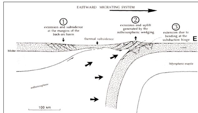
Figure 8. structural model of how the tensile range in a pressure system (Doglyuny 1995)
