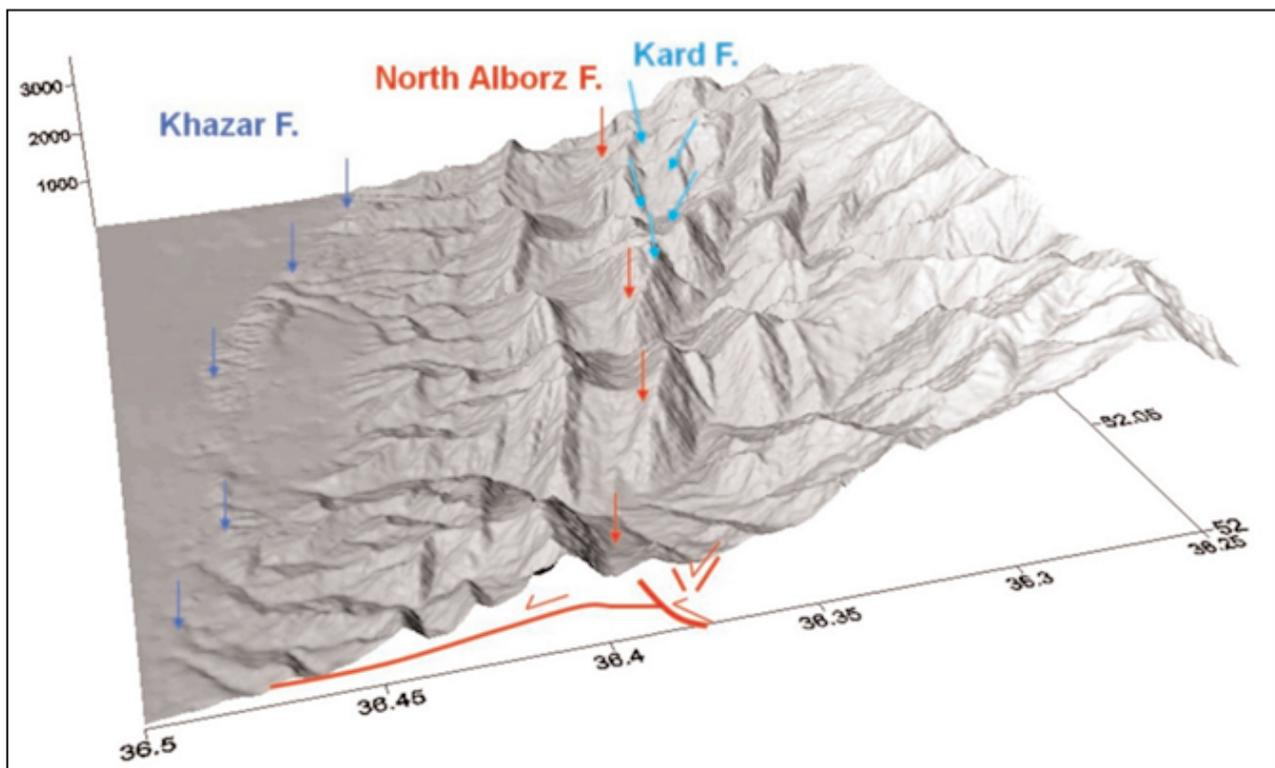
Figure 17. schematic model and structural relationship of North Alborz fault (red arrows), fault of Caspian (blue arrows) and stretching fault of Kard (turquoise arrows) on the wall of fault of north Alborz on a field of digital height model provided from topographic maps in scale 1:50000 in Chamestan area (west of Amol), which represents the progressive structures of fold and fault to the north. (Jahandar, 2014)
