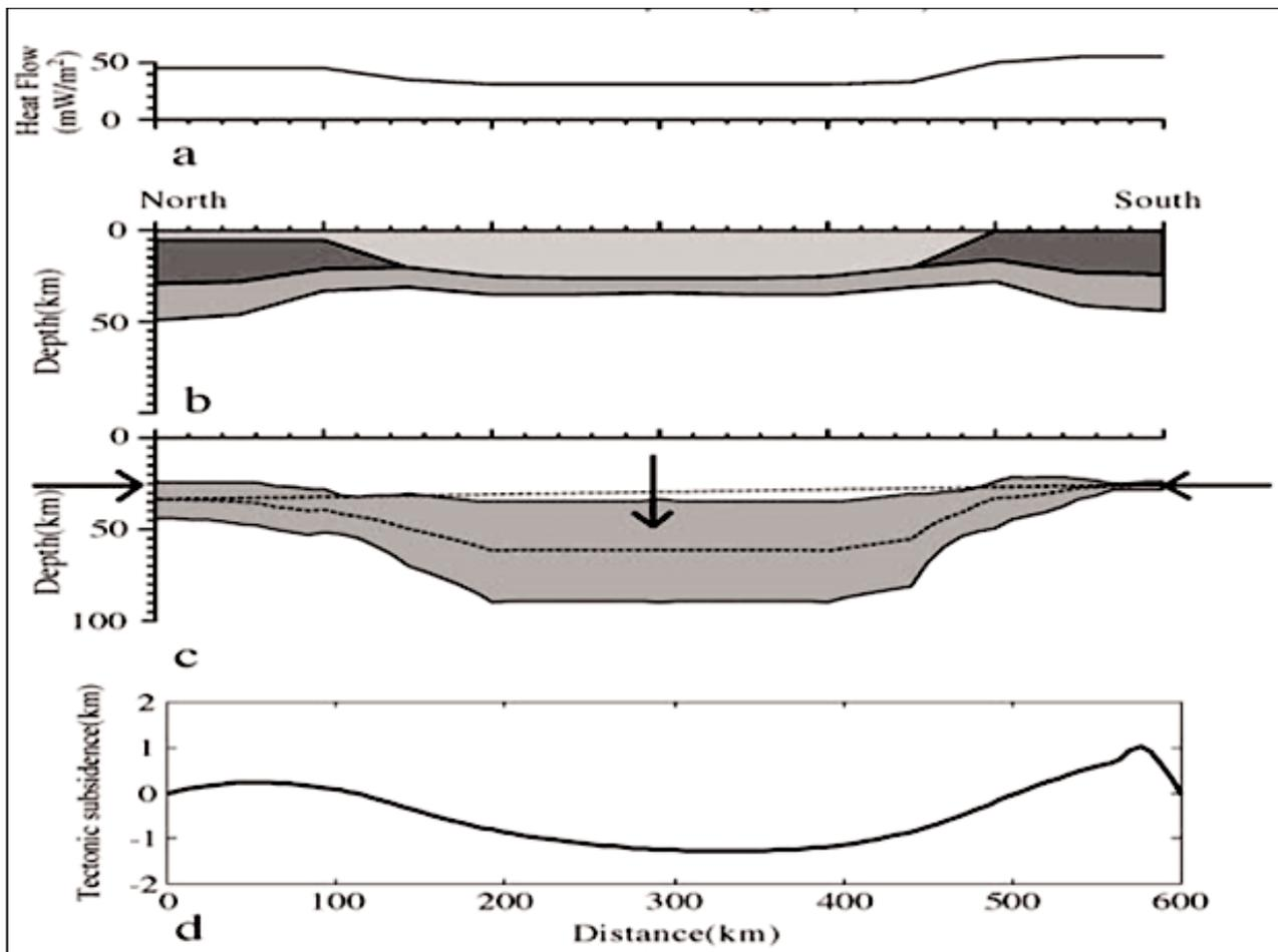
Figure 3. South Caspian basin subsidence model as bending downward due to performance of compressional forces, along with loading on the edges of the basin (Brent et al. 2003)
