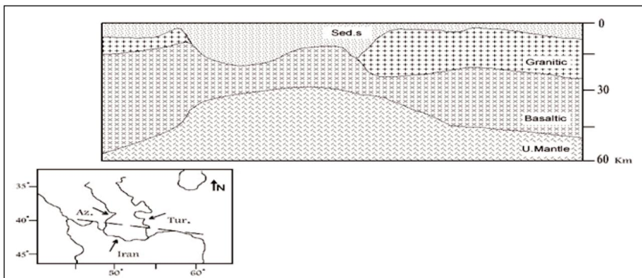
Figure 2. cross-section of the crust and the upper part of mantle in contour of Kura Basin in West of Caspian Basin
