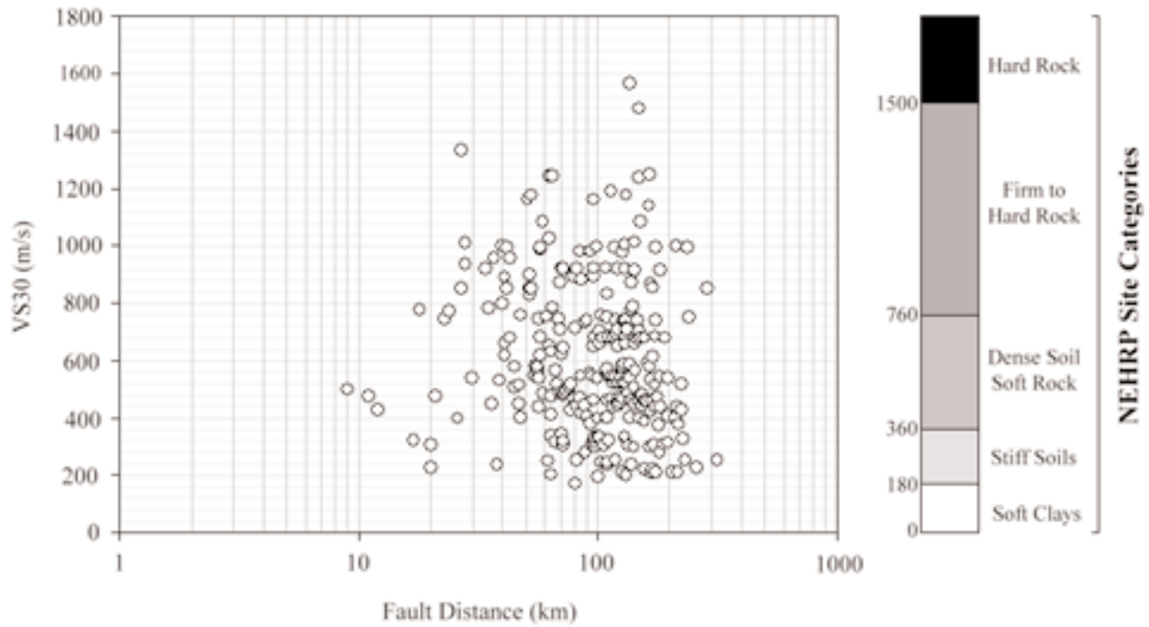
Figure 4. Earthquake data distribution with respect to VS30 and its comparison with NEHRP site categories.
