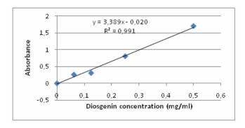
Figure 1 Calibration curve of standard diosgenin for determination of saponins content
