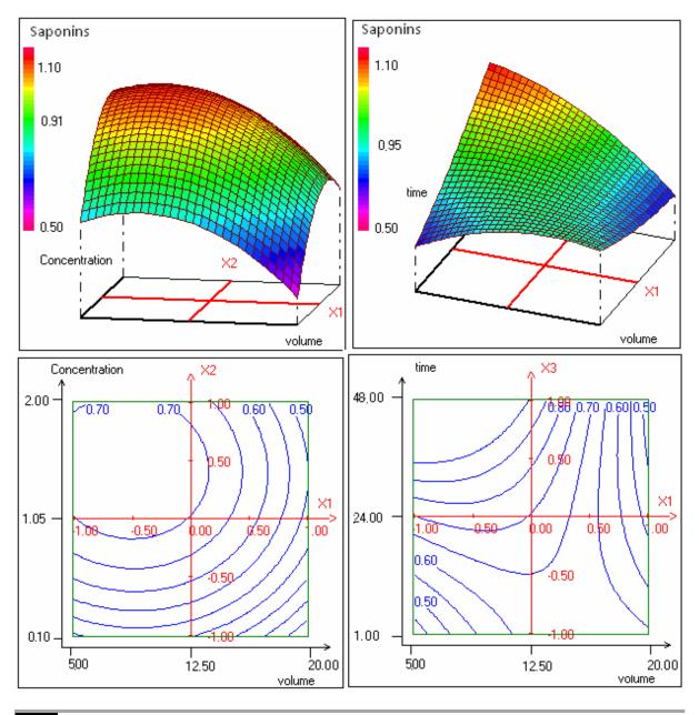
Figure 4 Response surface and contour plots showing the effect of soaking in citric acid on the levels of saponins from argane press cake
