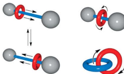
**Fig. 1.** Catenane and rotaxane in molecular machines
