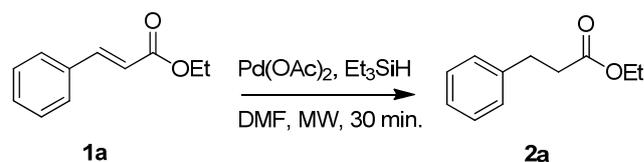
**Scheme 1.** Pd-catalyzed chemoselective 1,4-reduction of aromatic  $\alpha,\beta$ -unsaturated esters.
