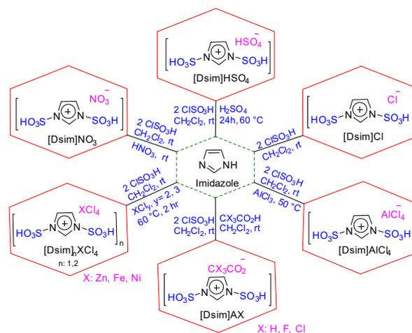
Scheme 1. The preparation of various form of [Dsim]X.
