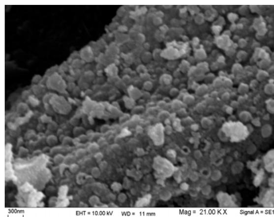
**Fig. 3.** SEM image of the obtained  $\text{ZnFe}_2\text{O}_4$  MNPs.
