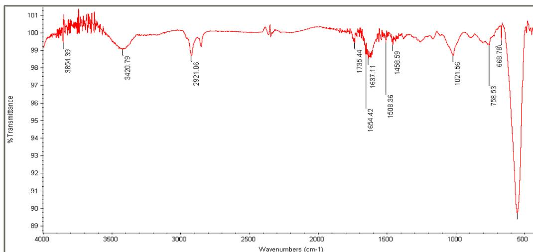
**Fig. 1.** FTIR spectrum of  $\text{ZnFe}_2\text{O}_4$  MNPs.
