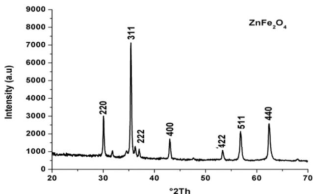
**Fig. 2.** XRD pattern of  $\text{ZnFe}_2\text{O}_4$  MNPs.
