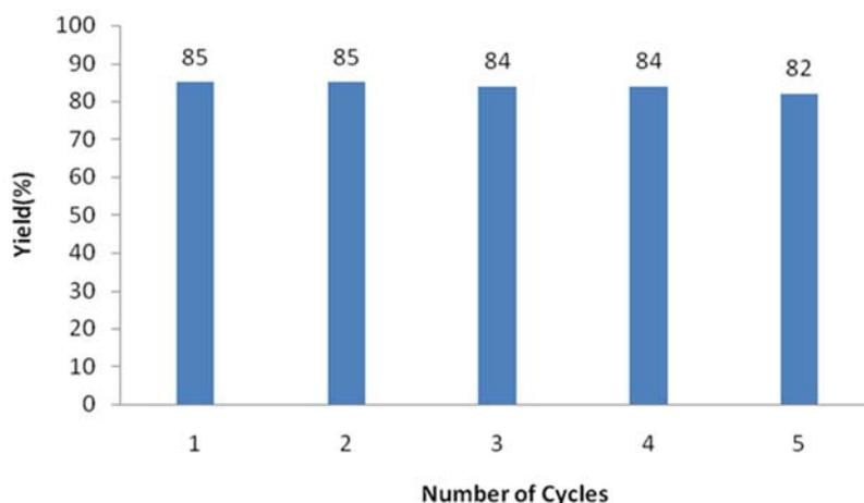
**Fig. 4.** Recycling of the catalyst for the oxidation of 4-chlorobenzyl alcohol.
