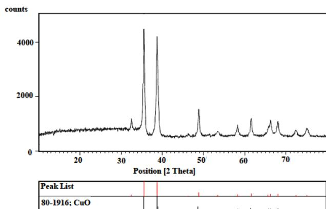
**Fig. 2.** The XRD pattern of CuO NPs.
