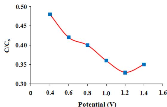
**Fig. 9.** PEC removal of 2,5-dichlorophenol as affected by the applied potentials on PEC degradation of 7.0  $\text{mg L}^{-1}$  2,5-dichlorophenol in phosphate buffer solution (pH 6.0) over experimental time 60 min.
