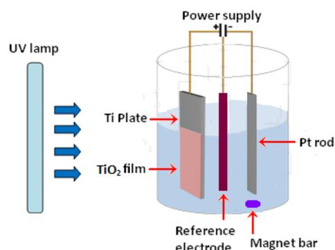
**Fig. 1.** Schematic of the photoelectrocatalytic batch reactor set-up.
