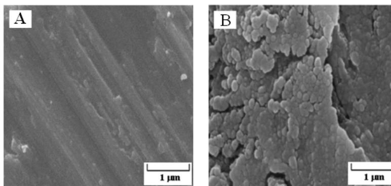
Fig. 2. A typical SEM micrographs of (A) Ti and (B) TiO<sub>2</sub>/Ti electrodes.
