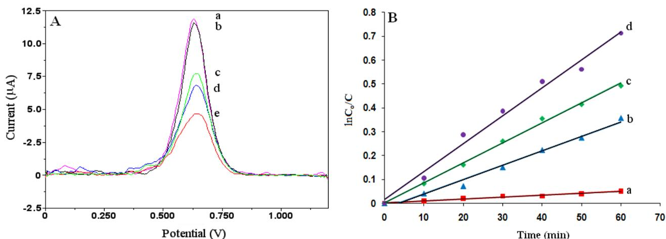
**Fig. 6.** A) Differential pulse voltammograms of 7.0 mg L<sup>-1</sup> 2,5-dichlorophenol at the TiO<sub>2</sub>/Ti electrode surface before (a) and after (b) EC, (c) DP, (d) PC and (e) PEC degradation processes, in 0.1 M phosphate buffer solution (pH 7.0) and E = 0.4 V vs Ag/AgCl/KCl (3M). B) Comparison of (a) PEC, (b) PC, (c) DP and (d) EC degradation of 2,5-dichlorophenol based on plot of lnC<sub>0</sub>/C as a function of time.
