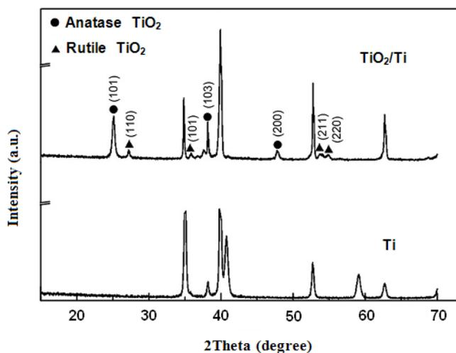
Fig. 3. XRD patterns of Ti and TiO<sub>2</sub>/Ti electrodes.
