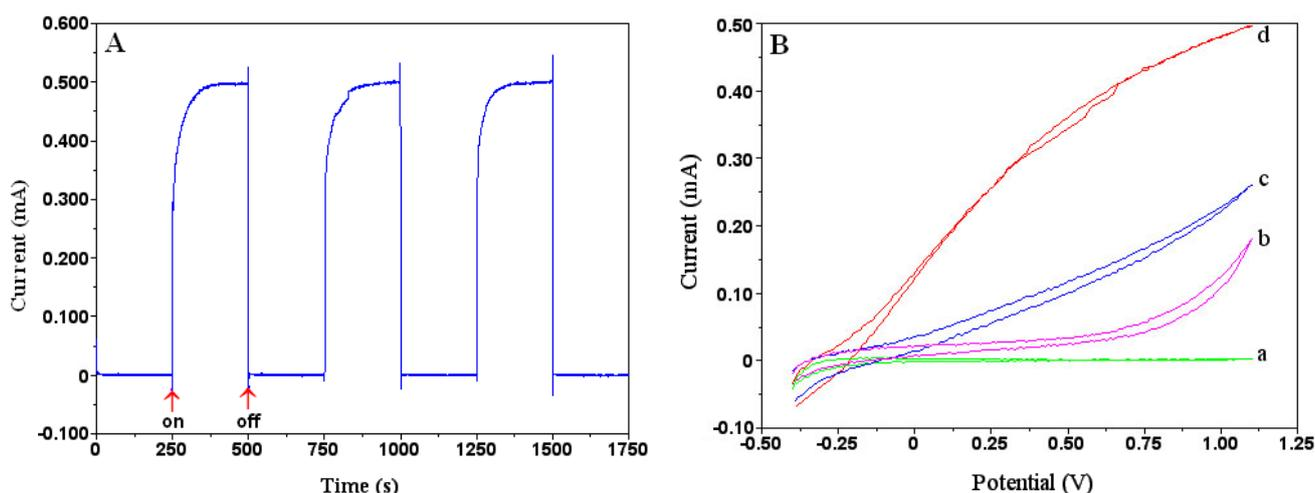
**Fig. 5.** A) Photocurrent-time response of TiO<sub>2</sub>/Ti electrode at a biased potential of 0.5 V vs. reference electrode under on-off cycles of irradiation in 0.1 M phosphate buffer solution (pH 7.0). B) Cyclic voltammograms of 70 mg L<sup>-1</sup> 2,5-dichlorophenol at the unmodified Ti electrode surface (a) in dark and (b) under UV irradiation, (c) and (d) as a and b at the TiO<sub>2</sub>/Ti electrode surface respectively at a scan rate 10 mV s<sup>-1</sup>.
