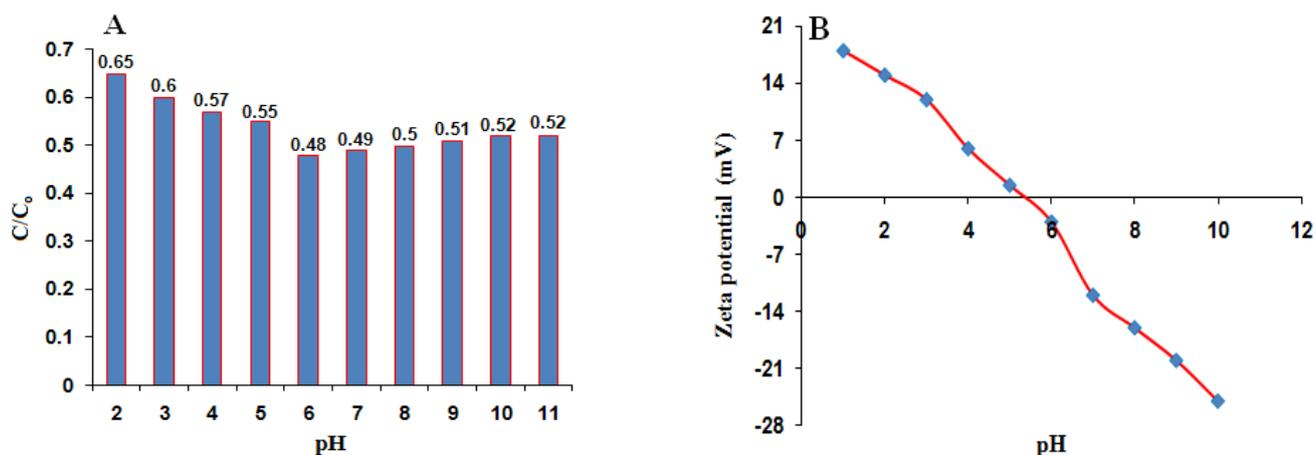
**Fig. 7.** A) Influence of pH on PEC removal of  $7.0 \text{ mg L}^{-1}$  2,5-dichlorophenol at the  $\text{TiO}_2/\text{Ti}$  electrode surface with bias potential  $0.4 \text{ V}$  vs  $\text{Ag}/\text{AgCl}/\text{KCl}$  (3M) over 60 min illumination. B) The Plot of zeta potential for  $\text{TiO}_2$  nanoparticles suspended in phosphate buffers as a function of the pH of the suspension.
