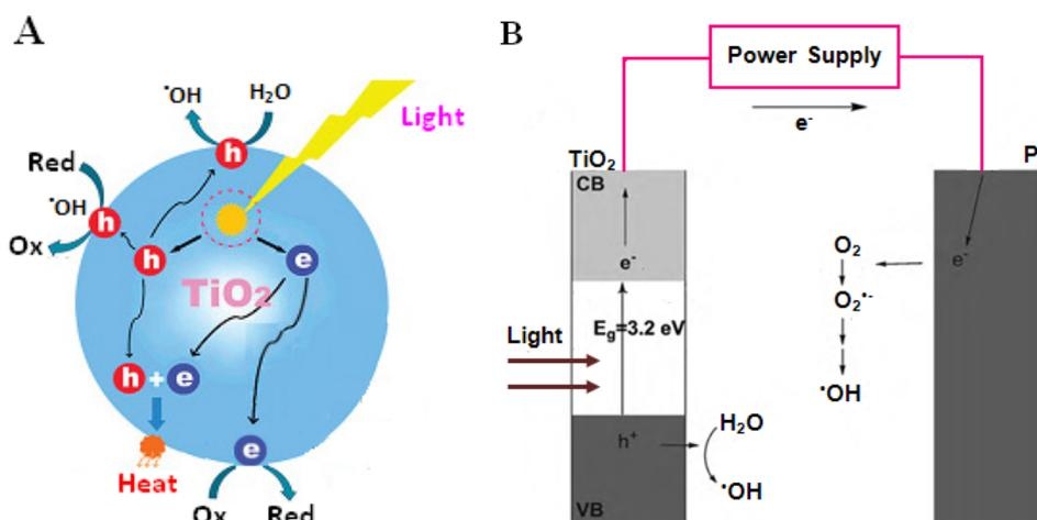
Fig. 4. Schematic photoexcitation, recombination and reaction processes of a semiconductor particle (A) and effect of applied potential on separation electron-hole at the surface of the TiO<sub>2</sub>/Ti electrode in photoelectrocatalysis process (B).
