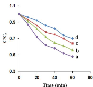
**Fig. 8.** Effect of the different initial 2,5-dichlorophenol concentration on its removal: (a) 7.0, (b) 9.0, (c) 11.0 and (d) 13.0  $\text{mg L}^{-1}$  in phosphate buffer solution (pH 6.0) on a  $\text{TiO}_2/\text{Ti}$  electrode with bias potential 0.4 V vs  $\text{Ag}/\text{AgCl}/\text{KCl}$  (3M).
