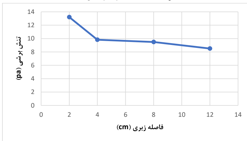
Fig 14. Changes in average bed shear stress
