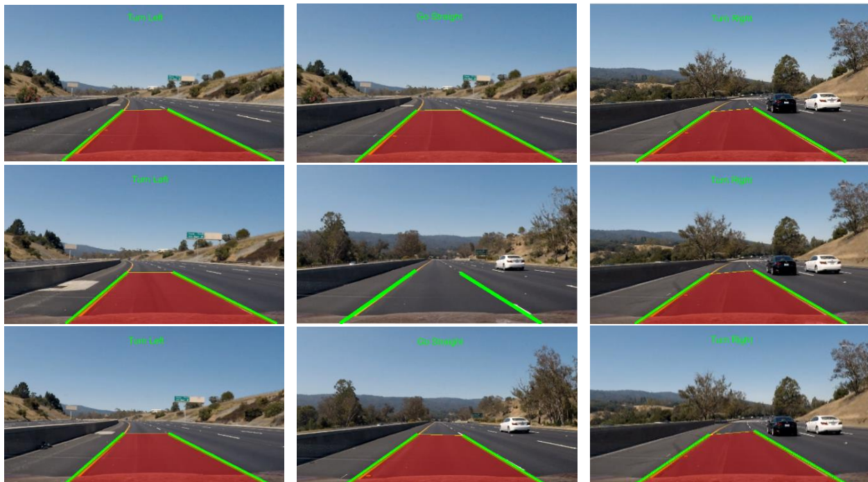
Fig. 3. lane line detection with proposed method.
