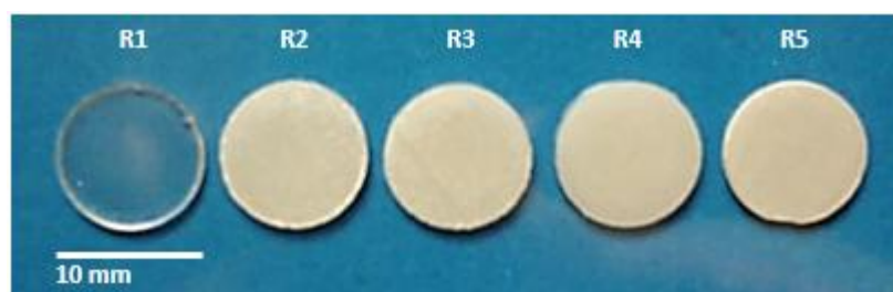
Fig. 1 Experimental adhesive disks: R1 (unfilled resin), R2 (20% CNC), R3 (15% CNC+ 5%ACP), R4 (20% ACP), R5 (40% ACP+5% CNC)
