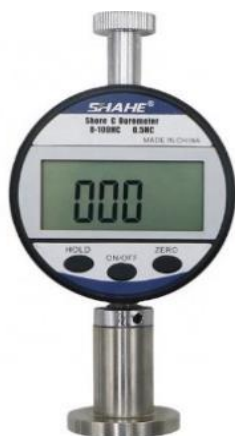
Fig. 6 Shore C stiffness tester.
