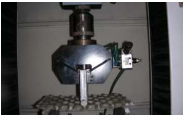
Fig. 4 Three-point bending test of composite grid panel.
