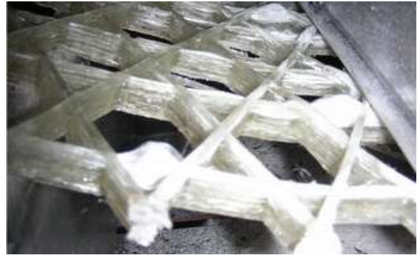
Fig. 8 Fiber buckling in the upside layers of the panel. The final structural failure was not possible due to the limitations of the test device displacement and the maximum force exerted by the tolerance of the fixture.
