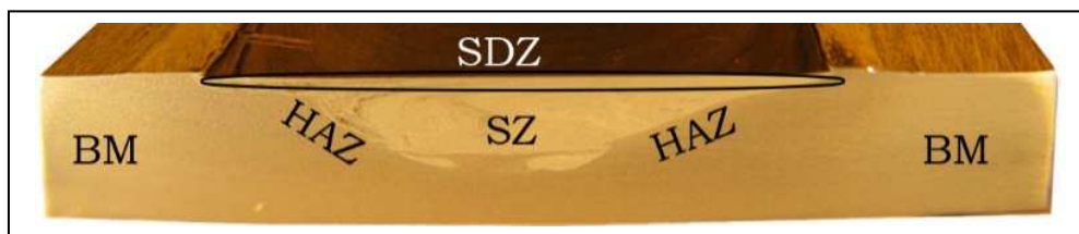
Figure6. Cross section of Al 6061/TiB 2 sample showing various microstructural zones
