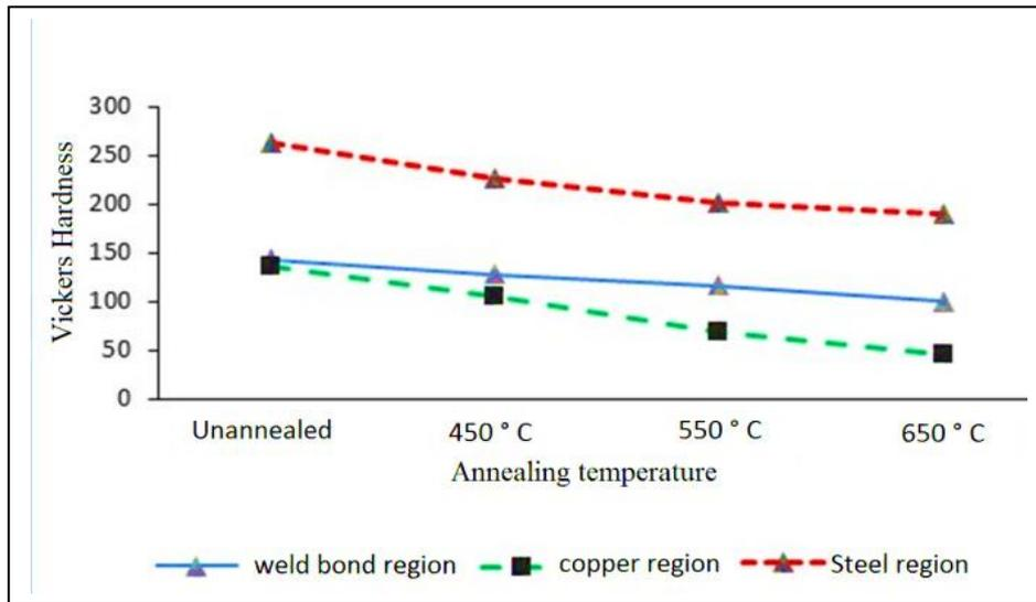
Figure3. The hardness of the two-layer sheet in different regions and annealing temperatures
