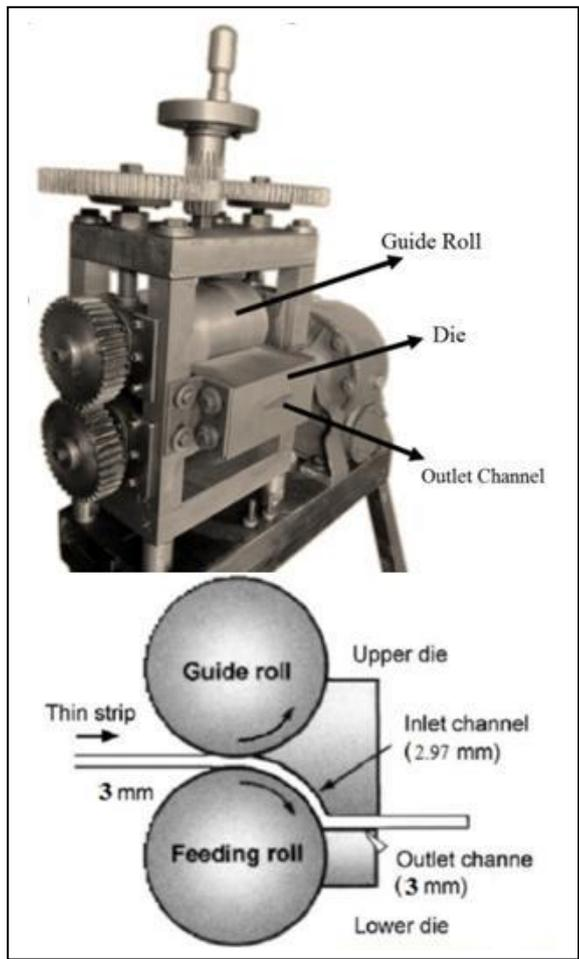
Figure1. The used device in this study, along with a schematic of the ECAR process
