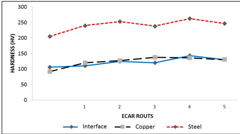
Figure2. The hardness of the two-layer sheet in various passes
