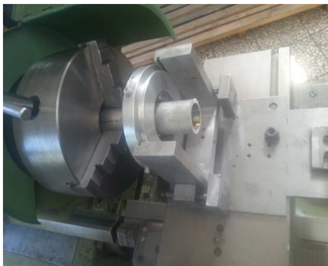
Figure4. Setup of magnetic abrasive finishing of inner surface
