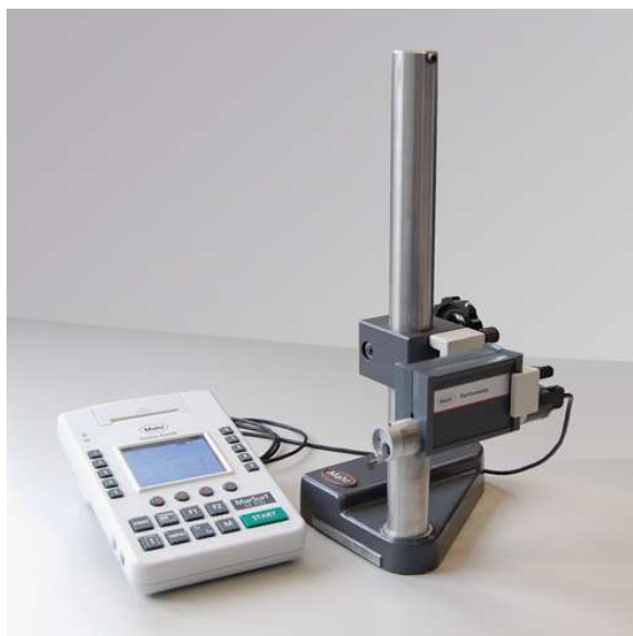
Figure2. The tool used for surface roughness measurement
