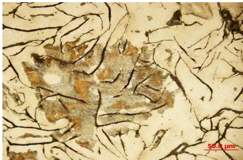
Figure4. Graphite sheets in sample ferrite-perlite structure taken from the pump impeller (affectation picral affectation)
