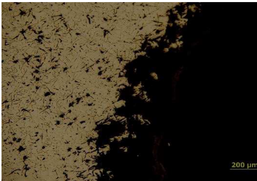
Figure8. Separation of cast iron from iron and leaving the black graphite layers on the surfaces of the pump impeller, when polishing the sample
