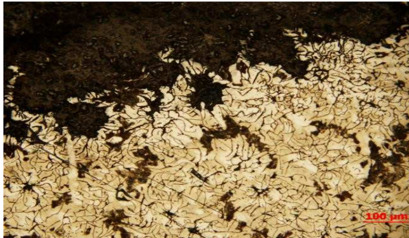
Figure9. Iron-free areas because of graphite corrosion
