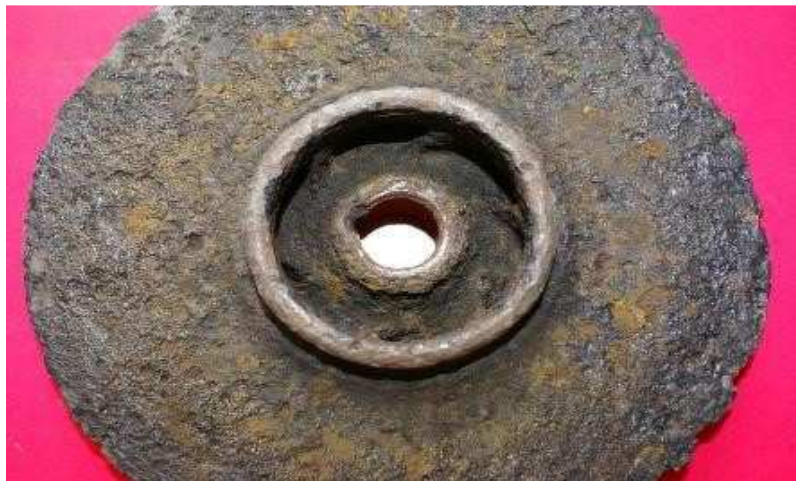
Figure6. Corrosion and destruction of water pump impeller of the cooling system air compressor
